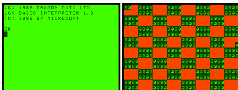
Figure 5.1: Emulator with and without BASIC ROM
